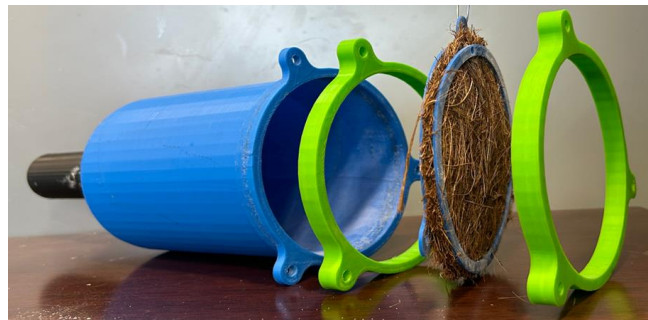
Figure 5: Prototype 3D printed device for testing purposes with fiber plate.
